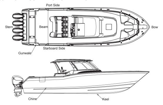
Abeam: a line perpendicular to a boat's keel
